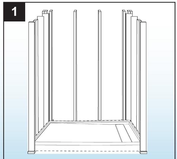
2. After applying the thin-set, replace the shims (if necessary) in the proper location and set the pan into place. Make sure the pan is resting level on the thin-set and shims and centered in opening.
