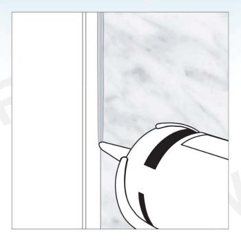
F. A small amount of silicone should be applied around the back of each plumbing hole penetration.
