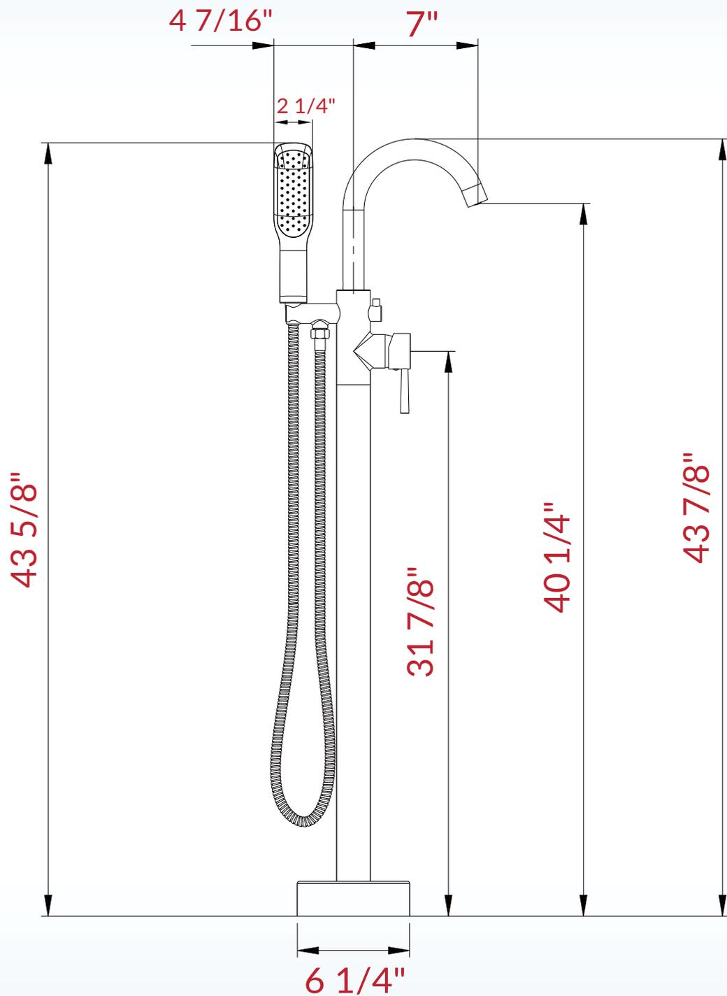
**ATTENTION!** Dimensions may vary by up to  $\frac{3}{8}$ ". It is highly recommended to pull all dimensions of actual model for installation and measuring purposes.
