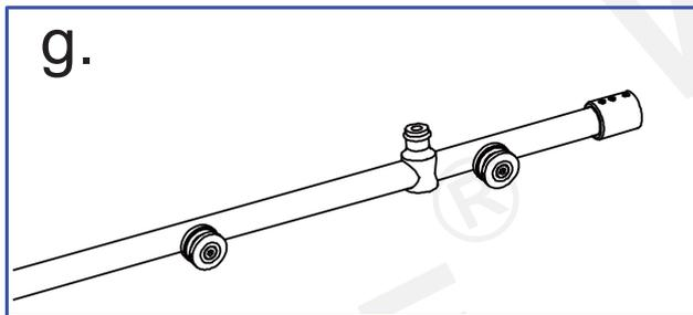
3. Use the Allen Key (19) to loose the screw on the Guide Rail Brackets (1) and Glass Door Stoppers (2). Slide the Glass Door Stopper and then the Guide Rail Bracket to the Guide Rail (3), use the Allen Key to tighten the parts to the guide rail temporarily.
