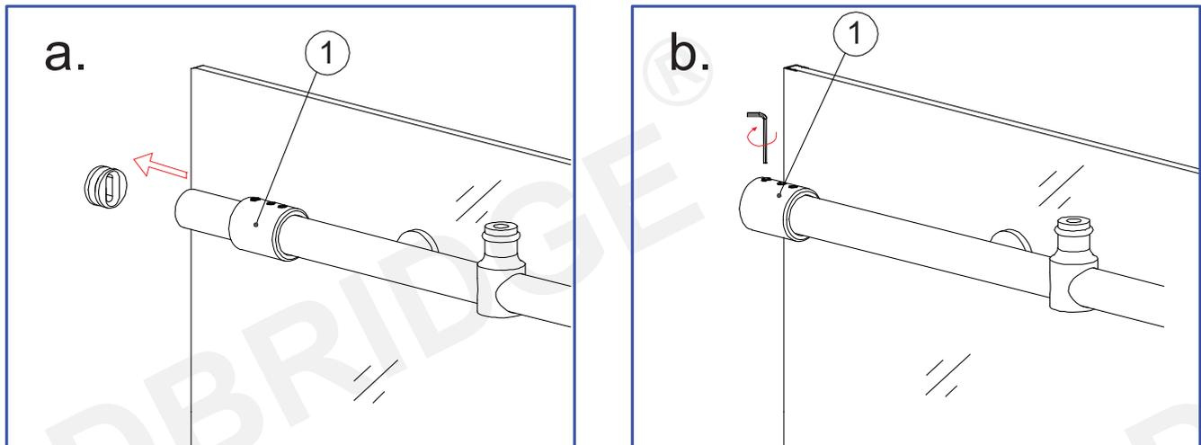
Note: The other side of the Guide Rail bracket (1) is installed in the same way.
