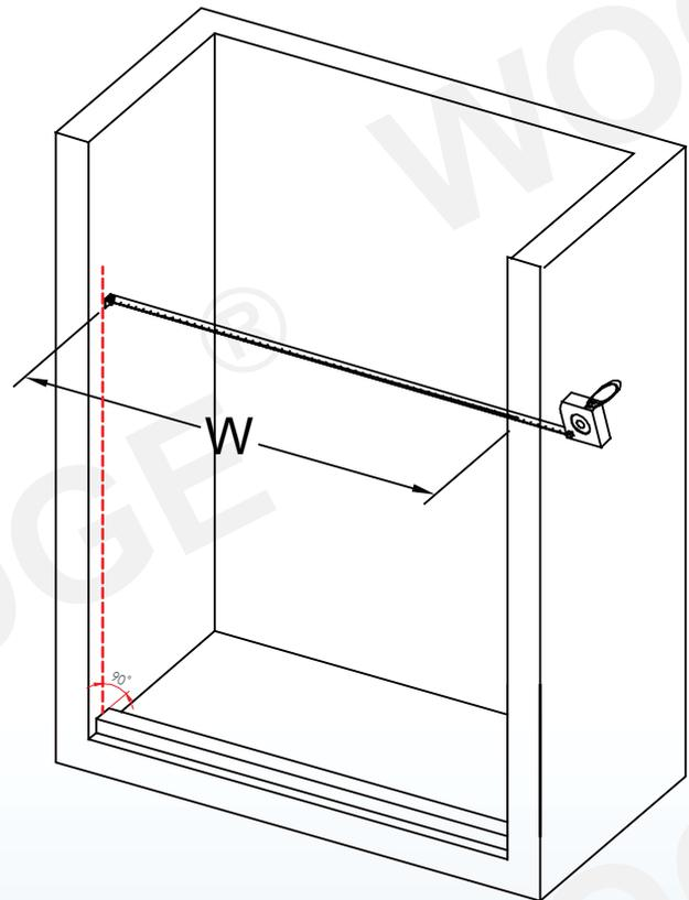
1. Measure the distance between two finished walls. This distance is marked as W.
