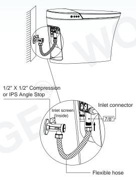
Connect the water inlet and angle valve of the toilet with the matching hose and tighten it
