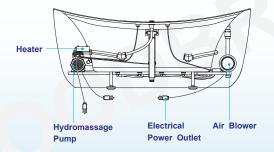
Built-in heater for consistent water temperature
