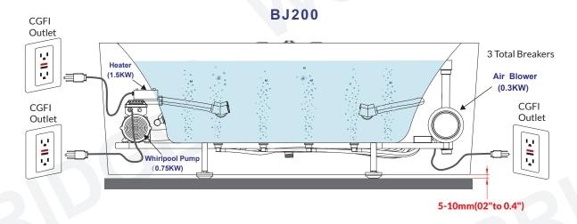
For Air Bath and Whirpool Tub installation, Do not apply any silicone sealant after installation, leave a 5-10mm(0.2" to 0.4")gap for motor/pump ventilation purpose.
