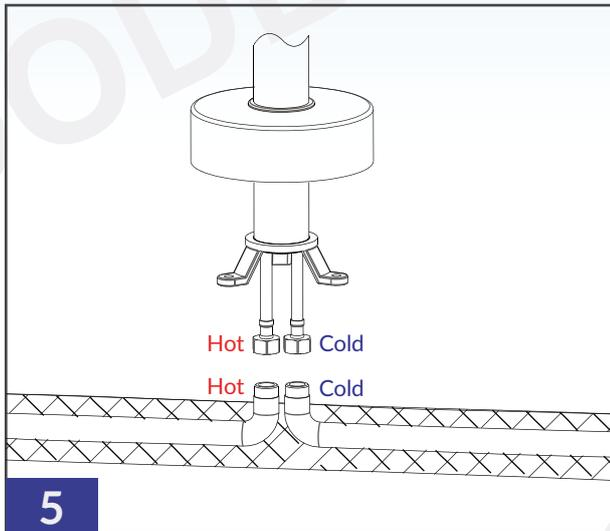
Step 5: Locate the faucet assembly onto the rough valves from floor, and secure the connection of inlet supply lines to the valves. **DO NOT** reverse the Hot and Cold supply.
