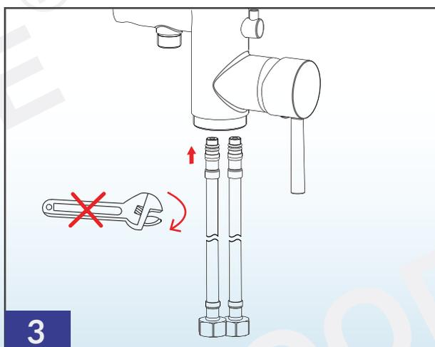
Step 3: Hand tighten the hot and cold flexible water supply line onto faucet body.
