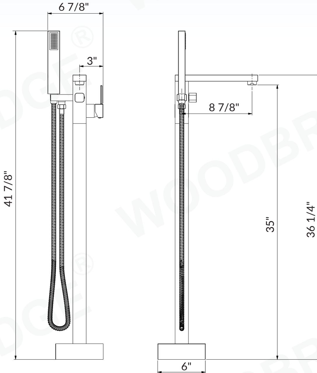
**ATTENTION!** Dimensions may vary by up to 3/8". It is highly recommended to pull all dimensions of actual model for installation and measuring purposes.
