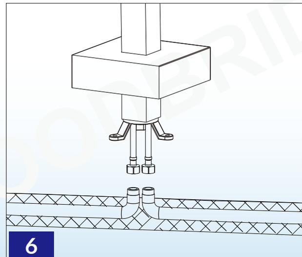
Connect another side of the flexible hose to the water supply pipe. Make sure they are to be fitted into the correct outlets for hot water and cold water.
