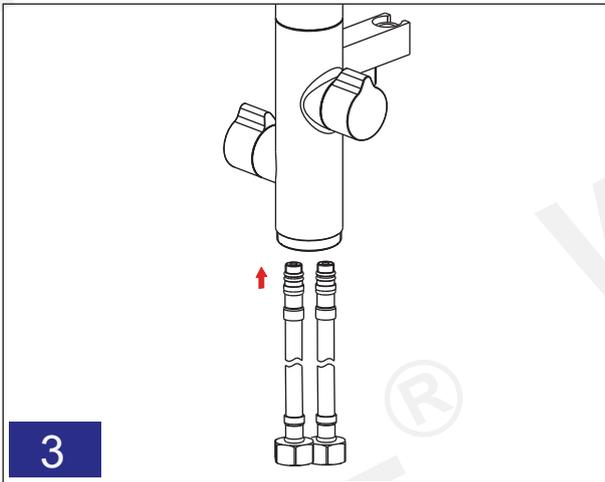
**3** Install the flexible hose now and ensure the flexible hoses are hand tightened into place. (DO NOT USE SPANNER TO TIGHTEN AS IT CAN DAMAGE THE O-RING). The flexible hoses are to be fitted into the correct inlets for hot water and for cold water.
