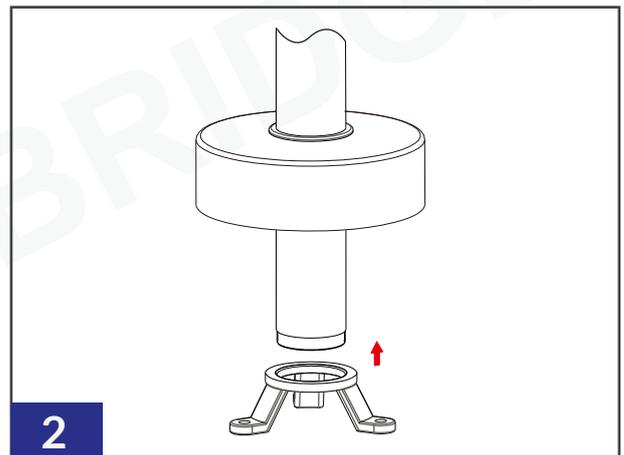
Step 2: Thread the tube onto the Triangle Pod.
