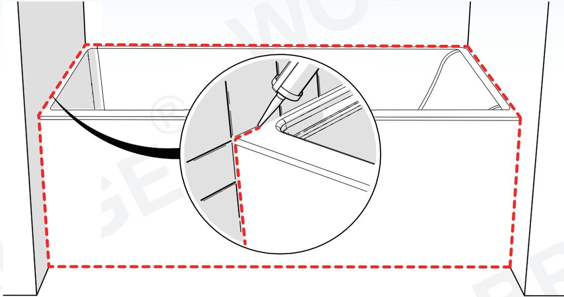
Reference for Correct Tile Flange Installation . Use drawing below as a reference guide for rough-in measurements.
