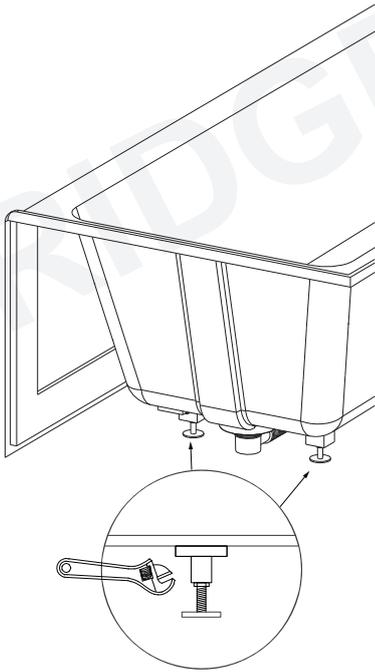
Lock the adjustment by tighten the hexagon nut.
