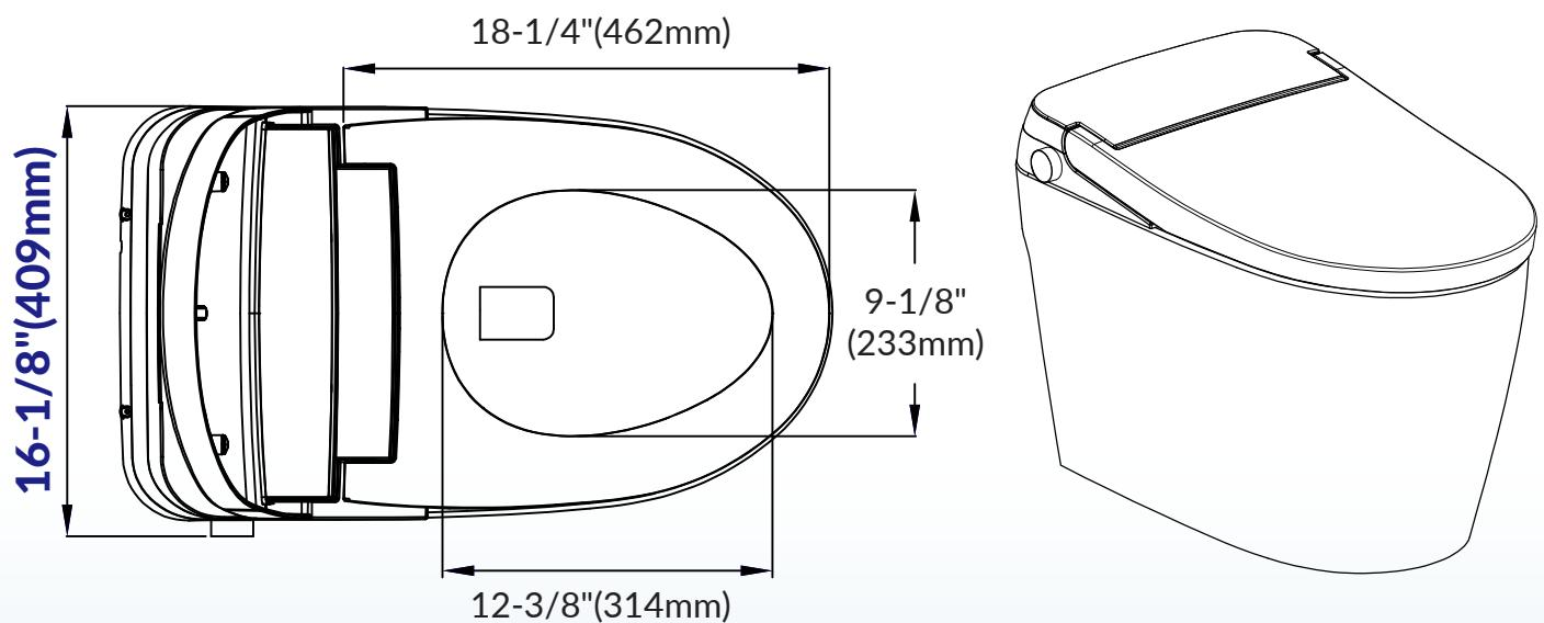
**ATTENTION!** Dimensions may vary by up to 3/8". It is highly recommended to pull all dimensions of actual model for installation and measuring purposes.
