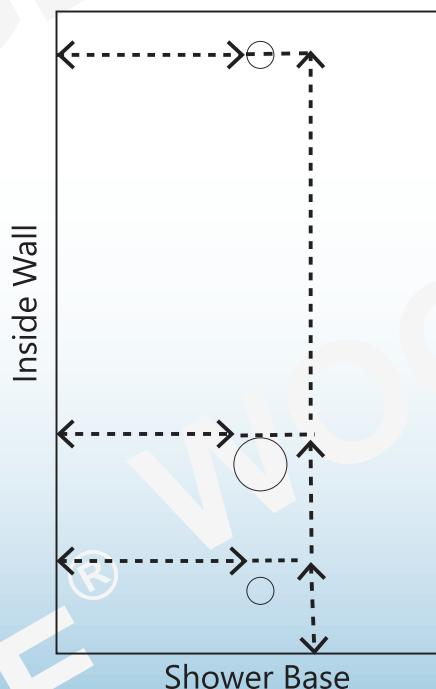
**NOTE: You will be able to make smaller adjustments to the panel for a more accurate fit after the holes are cut and your panel can be firmly pushed into the corner. Keep in mind the size and coverage of the trim kit and escutcheons.**
