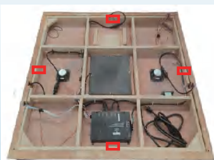
After connecting the power cable, the position of the frame is fixed with ST 4*40mm*4pcs screws.
