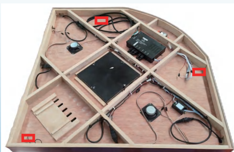
17. Installation of dust cover plate: put the power cable through the hole reserved in the dust cover plate, and use ST3.5*15MM*8pcs screws to fix the dust cover plate on the top plate.
