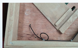
After connecting the power cable, the position of the frame is fixed with ST 3.5*40mm*3pcs screws
